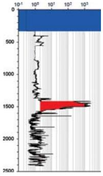
Borehole logging: For over 75 years, the primary method for determining the presence of hydrocarbons at various burial depths has been by using resistivity logs acquired with instruments delivered to the subsurface using wireline or while-drilling techniques. SBL now offers the opportunity for logging... without drilling.
