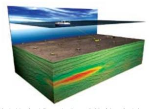
Seabed logging delivers subsurface resistivity information before drilling a well. Although the resolution is lower than from borehole logging or seismic imaging, the technique is an excellent "edge detector" and greatly improves reservoir delineation.
