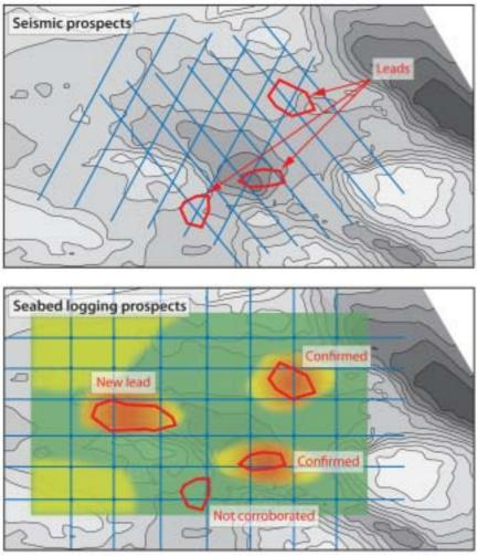
Improving the odds: A seismic survey (upper chart) indicates three areas where hydrocarbons may be found. Seabed logging (lower chart) confirms the presence of hydrocarbons in the case of two of the three leads, the red hot spots, and highlights a fourth area worth investigating, which the seismic survey had missed. Falklands Oil & Gas recently announced its intention to assess over 100 seismic prospects in the South Atlantic in this manner
