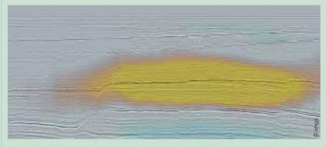
Depth migrated image from a one line survey across the giant Troll field in the North Sea. The reservoir is in Upper Jurassic sandstones situated below the prominent reflector in the middle of the section. The hydrocarbon filled reservoir at a depth of approximately 1000m has resistivities approaching 250  $\Omega$ m, while water wet sandstones and overburden shales have resistivities in the order of 1-2.5  $\Omega$ m.
