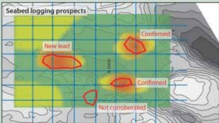
While seismic data define prospects and leads, seabed logging is capable of confirming the presence of hydrocarbons. In this example, two of three leads seem to be promising. A fourth area, which is missed by the seismic, should be pursued. The figure thus illustrates how seabed logging helps to prioritize an exploration campaign.
