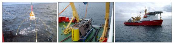
Figure 1: The left picture shows the first instrument dropped over Ormen Lange. All instruments have electrodes mounted at the end of each electrode arms, with lengths around 8m, giving two orthogonal electrical channels. The electric field measured at each channel is amplified and converted from analog to digital format before being recorded on an internal storage device. The EM source tow fish is displayed in the middle. The Polar Bjørn shown to the right was used as survey vessel.
