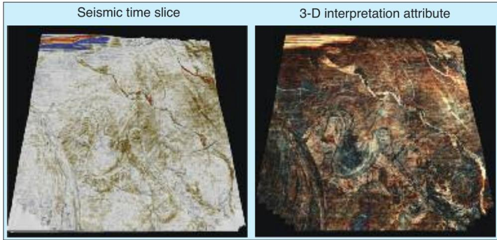
Example of IsoMetrix data aiding overburden resolution: A seismic time slice and equivalent slice from a colored 3-D interpretation volume extracted along a shallow dipping horizon show fine detail in channel systems. (Image courtesy of WesternGeco, a Schlumberger company)
