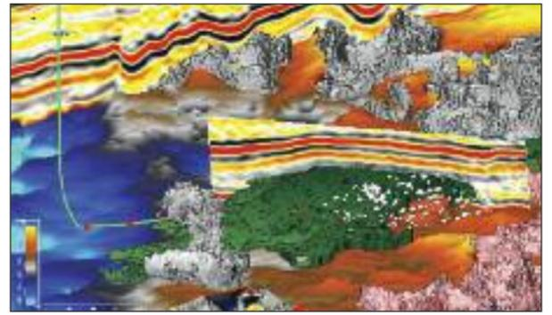
An integrated display of data in the Barnett incorporates seismic data, horizons, geobodies, karsts, wells and microseismic data. (Image courtesy of Paradigm)
