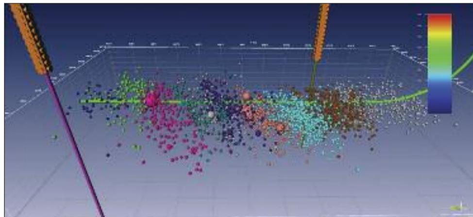
Integrated reservoir characterization workflows that enable real-time frack data and microseismic events to be processed, interpreted and visualized in tandem with the earth models, well geometries and geomechanical properties help operators know where to drill, where to frack and how to frack. (Image courtesy of SIGMA<sup>3</sup>)
