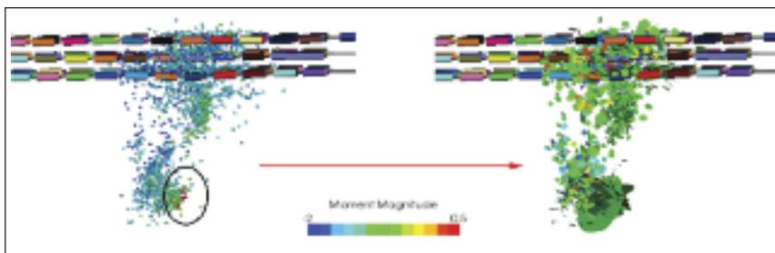
Figure 1. Microseismic events colored by moment magnitude are shown on the left. At right, a microseismic-derived discrete fracture network was obtained using data from a hybrid sensor network. Larger magnitude seismic events represent considerably larger fracture surface areas and result in more energy release and reservoir deformation compared to typical microseismic events. (Image courtesy of ESG Solutions)
