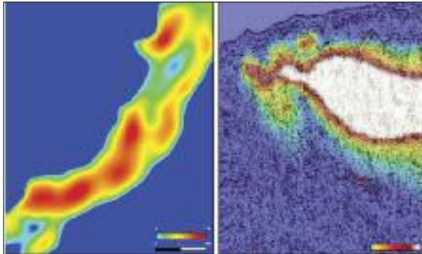
A Wilcox resistivity map (left) and an improved salt body interpretation (right) show data from the Daybreak survey in Alaminos Canyon in the GoM. (Data courtesy of TGS)
