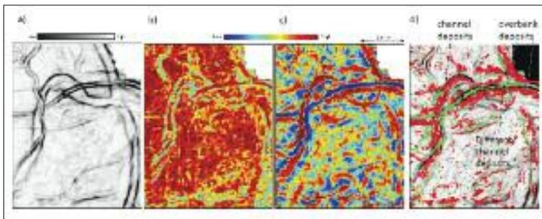
Stratal slice at a level close to a horizon picked at 1,020 ms from (a) coherence volume computed using the energy ratio algorithm, (b) GTM1, (c) GTM2 and (d) cluster points from the cross-plot of GTM1 and GTM2 attributes within two polygons—one in red and the other in green—that are projected onto the coherence stratal slice, highlighting different channels. (Image courtesy of Arcis Seismic Solutions and the University of Oklahoma)
