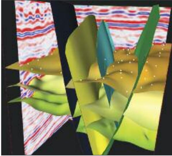
MDI enables users to not only create the geological model while conducting seismic interpretation but also to capture uncertainty while interpreting. (Image courtesy of Emerson Process Management)
