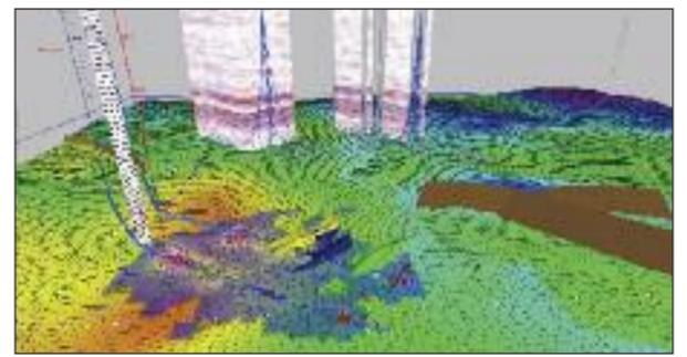
Using Weatherford's subsurface microseismic services, operators can see real-time hydraulic fracture monitoring and mapping to optimize well and fracture trajectories and avoid unanticipated subsurface complications. (Image courtesy of Weatherford)
