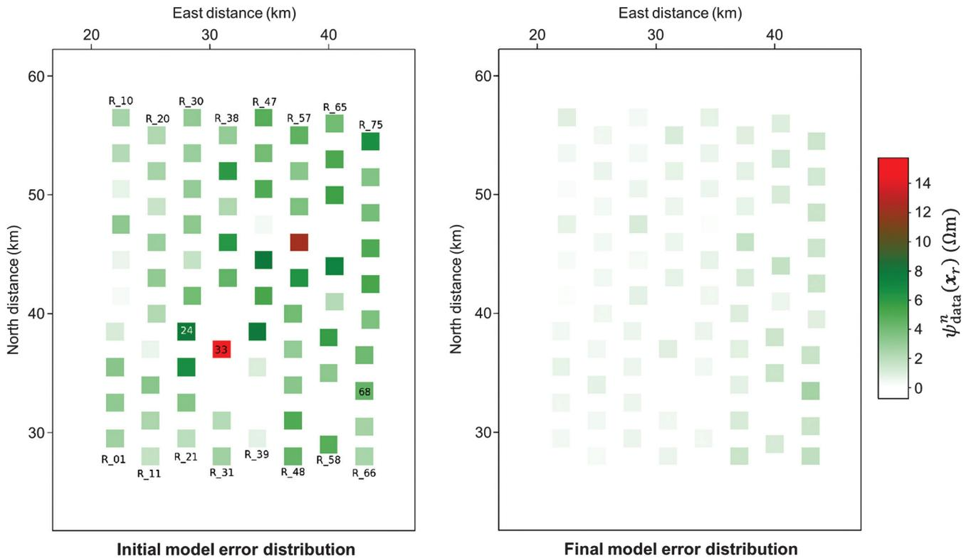
Figure 7. Data-space error  $\psi_{\text{data}}^n$  as a function of receiver location  $\mathbf{x}_r$  (see equation 27). The kernel of the misfit function can be viewed as a misfit in apparent resistivity. Hence,  $\psi_{\text{data}}^n$  is measured in  $\Omega\text{m}$ .
