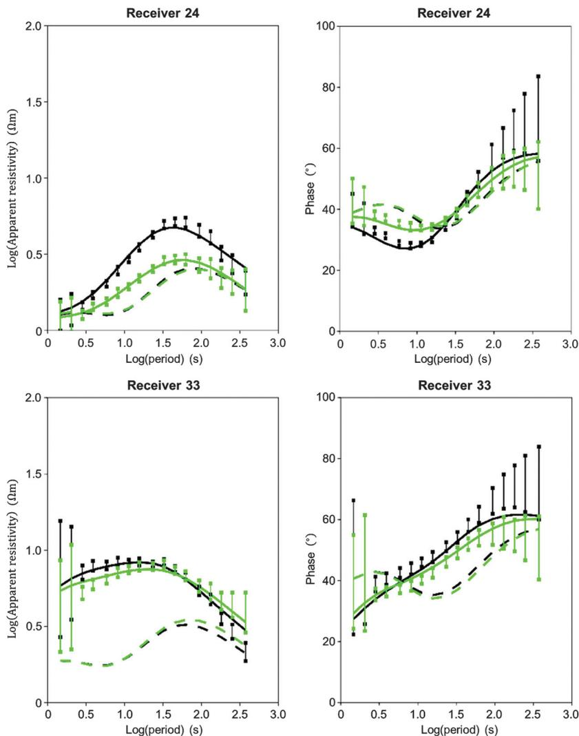
Figure 9. Apparent resistivity and impedance phase. The black lines are for  $Z_{xy}$ , and the green lines are for  $Z_{yx}$ . The observed data are displayed with error bars. The predicted data from the initial and final models are displayed with dashed and solid lines, respectively.
