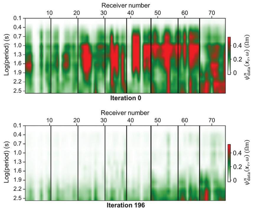
Figure 8. Data-space error  $\psi_{\text{data}}^n$  as a function of receiver location  $\mathbf{x}_r$  and period  $T = 2\pi/\omega$  (see equation 28), for the start model (top) and the model after the final inversion iteration (bottom). The kernel of the misfit function can be viewed as a misfit in apparent resistivity. Hence,  $\psi_{\text{data}}^n$  is measured in  $\Omega\text{m}$ .
