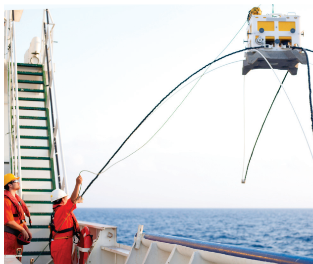
Figure 1: An EMGS crew deploying a sensor during an EM-imaging survey. The sensors, which measure electric and magnetic fields, sink to the ocean floor with the aid of an eco-friendly anchor. Upon survey completion, the sensors are released and retrieved at surface and the anchors remain on the ocean floor and dissolve into natural materials after a few months. Multiple sensors are positioned in a grid or linear pattern at distances ranging from one to five km, depending on the survey's objective.
