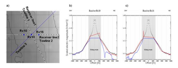
**Figure 2.** Bathymetry map with the survey layout. Black squares are receiver positions, solid lines are towlines. Receivers and corresponding towline discussed below are marked with blue (a). Figure b and c show Magnitude vs. Offset (MVO) for electric data at 1.0 Hz. Black circle is true inline data for receiver Rx13, red solid line is decomposed azimuth data and blue solid line is data prior to decomposition. Grey area indicates azimuth mute applied.
