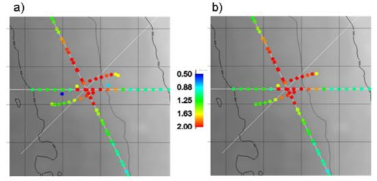
**Figure 3.** NMVO map at 4km source-receiver offset with true inline and decomposed data displayed together. No azimuth mute applied is shown in a, while data with azimuth angle larger than 50 degrees are muted in b. The two data types show consistent results and gives additional information to the survey.
