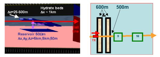
**Figure 2.** Left panel: illustration of hydrate patches with a characteristic length scale of  $\sim$ 1 km at a 1.7 km water depth above a synthetic target reservoir. Right panel: Top view of hydrate patches with the location of the receivers RX9 ("9") and RX 10 ("10") with 1.25km spacing.
