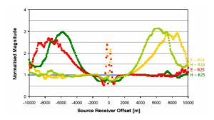
Figure 4: Normalized electric and magnetic magnitudes for receivers R16 and R25 for both in- and out-towing (0.25 Hz). Reference receiver is R41 out-towing.
