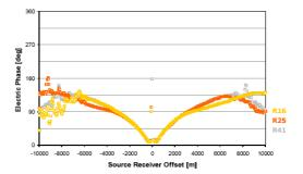
Figure 5: Electric phase versus source receiver offset for receivers R16, R25 and R41 for both in- and out-towing (0.25 Hz).
