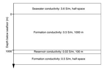
Figure 1. The plane-layered model used for comparison of results. The model consists of a semi-infinite water layer, a 1-km formation layer, a 100-m resistive layer, and a semi-infinite formation layer.
