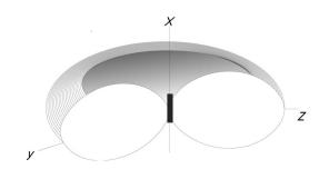
Figure B-1. Radiation pattern for the electric dipole. The radiation is symmetric around the dipole axis and largest normal to the dipole axis.
