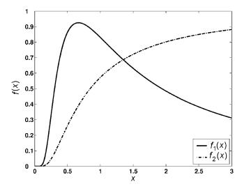
Figure 3. Step responses for dipole radiation in conductive materials: far-field response  $f_1(x)$  (solid line) and near-field response  $f_2(x)$  (broken line). The far-field response is largest for x < 1.4.
