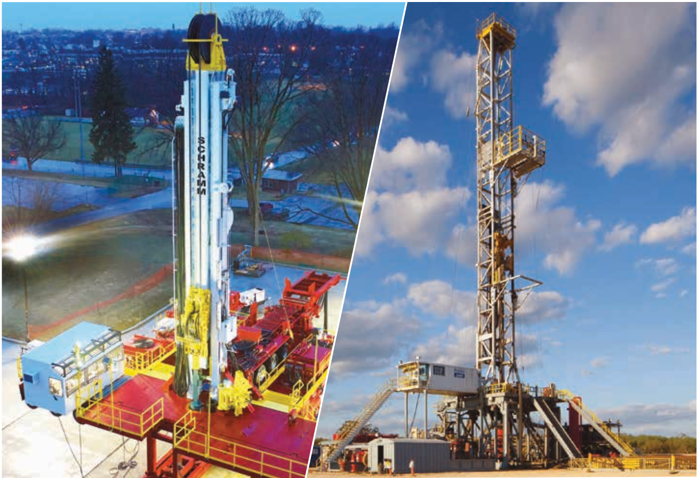
Figure 1. Left: MDR fully automated with 26 m rig-floor-to-top-of-mast height and no men on the floor or at height. Right: Equivalent class advanced AC Drive with 41 m height from floor to top. Men are required to work at height and on the rig floor.
