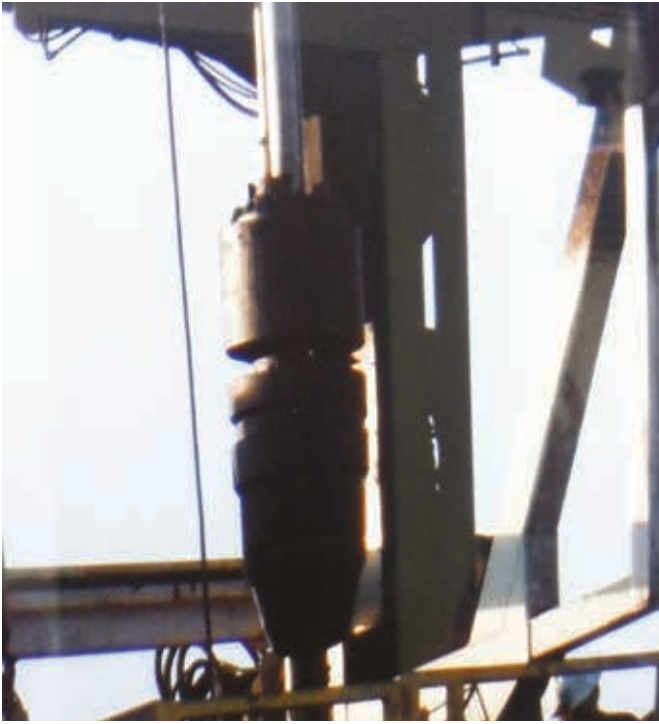
Figure 6. Dual element RCD bearing installing on a tool joint.
