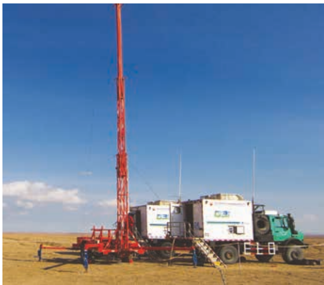
Figure 4. BGP utilised small recording trucks to house G3i's central and QC station computers.
