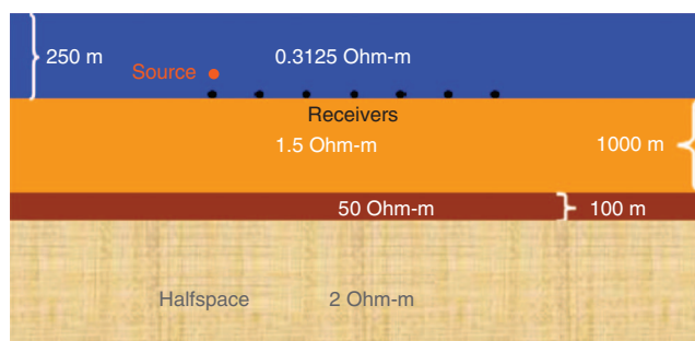
Figure 6. The cross-section of the shallow-water 3D resistivity (conductivity) model used for comparison to the plane-layer method.
