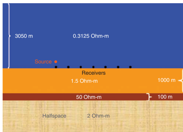
Figure 4. The cross-section of the deep-water 3D resistivity (conductivity) model used for comparison with the plane-layer method.
