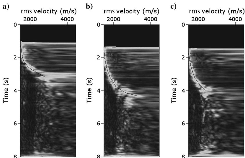
multiples that develop within the basalt sequence. SRME was successfully used to remove the seafloor-related multiples, and Radon-transform-based multiple attenuation techniques were used to attenuate the secondary multiples from the top-basalt interface. However, the intrabasalt multiples are difficult to eliminate due to the small velocity separation between the multiples and the primary reflections from within the basalt sequence.
