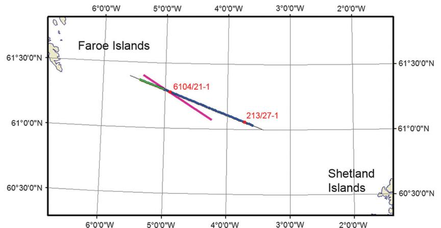
Figure 3. Map showing the location of the FLA\_06 seismic line (magenta line), the location of the CSEM and MT receivers used for this study, from the 2012 survey (blue dots), from the 2014 survey (green dots), and the CSEM tow line (thin black line). The locations of the Brugdan well (6104/21-1) and the Rosebank well (213/27-1) are also shown (red dots).
