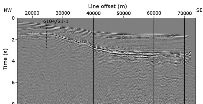
Figure 4. Time stack of the processed data. The location of the Brugdan well (6104/21-1) is indicated by the dashed black line. The solid black lines indicate the position of the semblance plots as shown in Figure 5.
