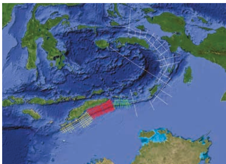
Figure 2. Google Earth image showing BandaSeis seismic survey components (Phase 1, West Timor, yellow; Phase 2, east of Timor, green; Phase 3, white; Phase 4, Timor Leste, red).
