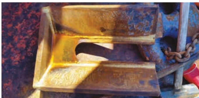
Figure 6. Custom made installation aide to extend the capability of the Shark Jaws.
