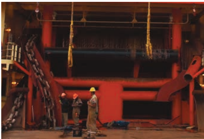
Figure 4. Chain handling on AHV Joshua Chouest. Note the modified chain chutes (in burgundy instead of dark orange), which routed the chain from the lockers to the whelps and back deck.
