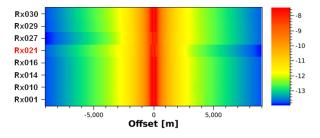
Figure 7: Synthetic MVO data,  $\log |E_{in}|$  at 0.1 Hz, computed using the model from Figure 6. Data for receiver Rx021 located on the trench slope shows a strong reduction in the magnitude on outtow and an increase on the intow, as compared to other receivers. These are the same trends as for real data of Rx080 in Figure 5.
