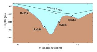
Figure 1: Seabed geometry, CSEM source trajectory and receiver positions (triangles) for a CSEM survey offshore Brazil.
