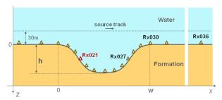
Figure 6: Bathymetry profile, source trajectory and receiver positions used for a synthetic study of the trench effect. Data for receiver Rx021 turned out to be most affected by the presence of the trench.
