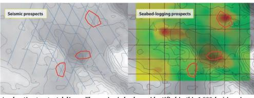
Accelerating prospect delivery: Three seismic leads are identified in this 1,000-km<sup>2</sup> imaginary frontier area (left). Scanning quickly confirmed two of the seismic leads and revealed a major new stratigraphic lead that had not been identified from seismic data (right). One of the seismic leads had no seabed-logging response. As it is unlikely to contain hydrocarbons, it can be dropped from the portfolio.
