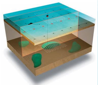
Focused exploration: Scanning data can be acquired using sparse grid patterns and evaluated quickly to identify, confirm, rank or exclude prospects. More detailed 2D or 3D seabed-logging surveys can then be designed and acquired to investigate prospects while the vessel is in the survey area, and the processed and interpreted data can be used to optimise well placement.
