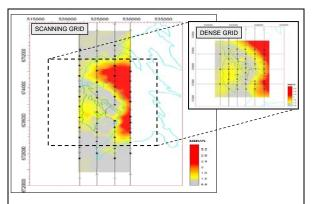
Figure 1: Receiver positions (black squares) and shot lines (gray) in scanning (left) and dense (upper right) grids. Normalized smoothed magnitudes (NMVO) are shown in color according to legend. The excitation frequency is 0.25 Hz, and data at an offset is 6.5 km were used. The reference receiver is the lowermost located one in the second line from left side. The western oil and gas zone is outlined in green (left) and the much larger eastern gas zone in blue.
