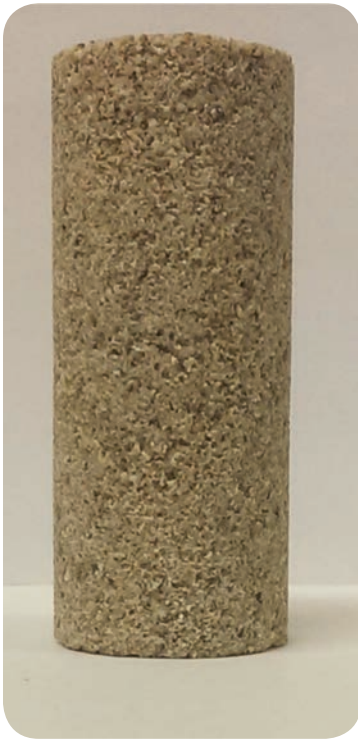
Above left: A 3D-printed core sample. Right: A 2D core sample visualization.
