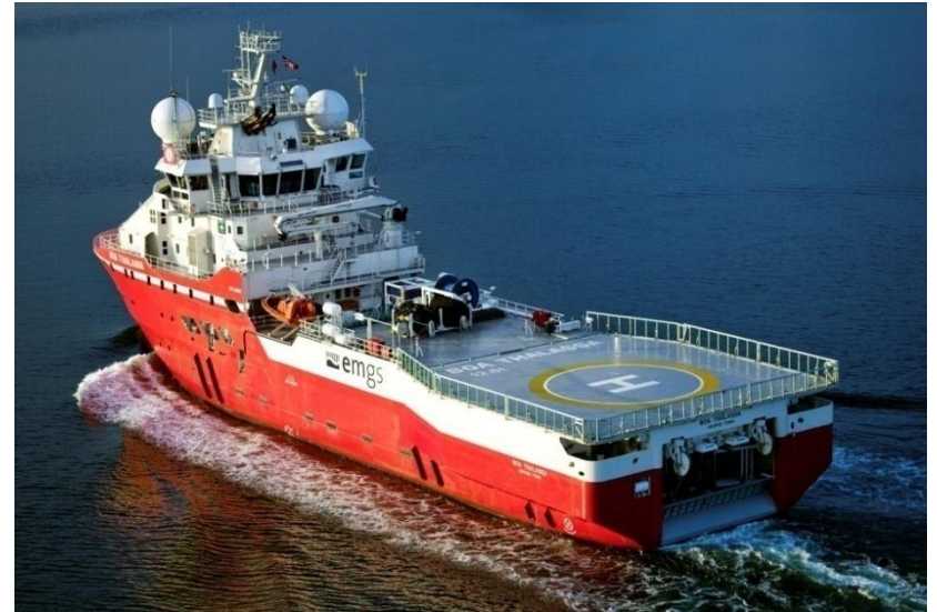
Purpose-built 3D EM vessel BOA Thalassa
