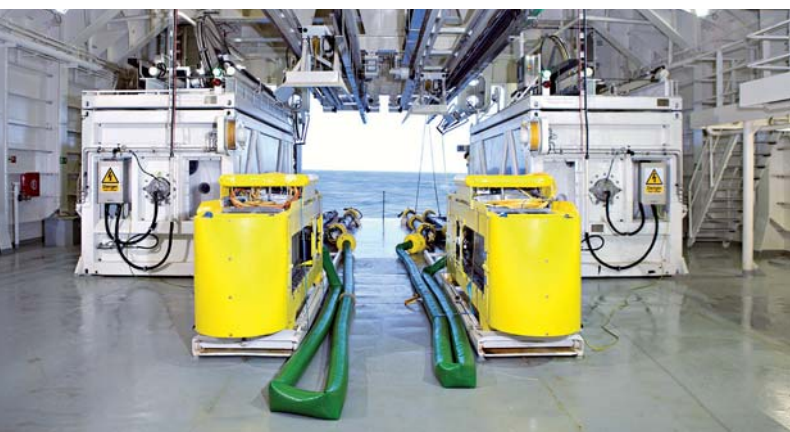
The vessel's fully integrated spare equipment set has two parallel source and receiver systems, including winches, cranes and hydraulic feeds.
