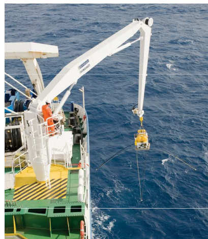
Receiver being deployed from multipurpose vessel
