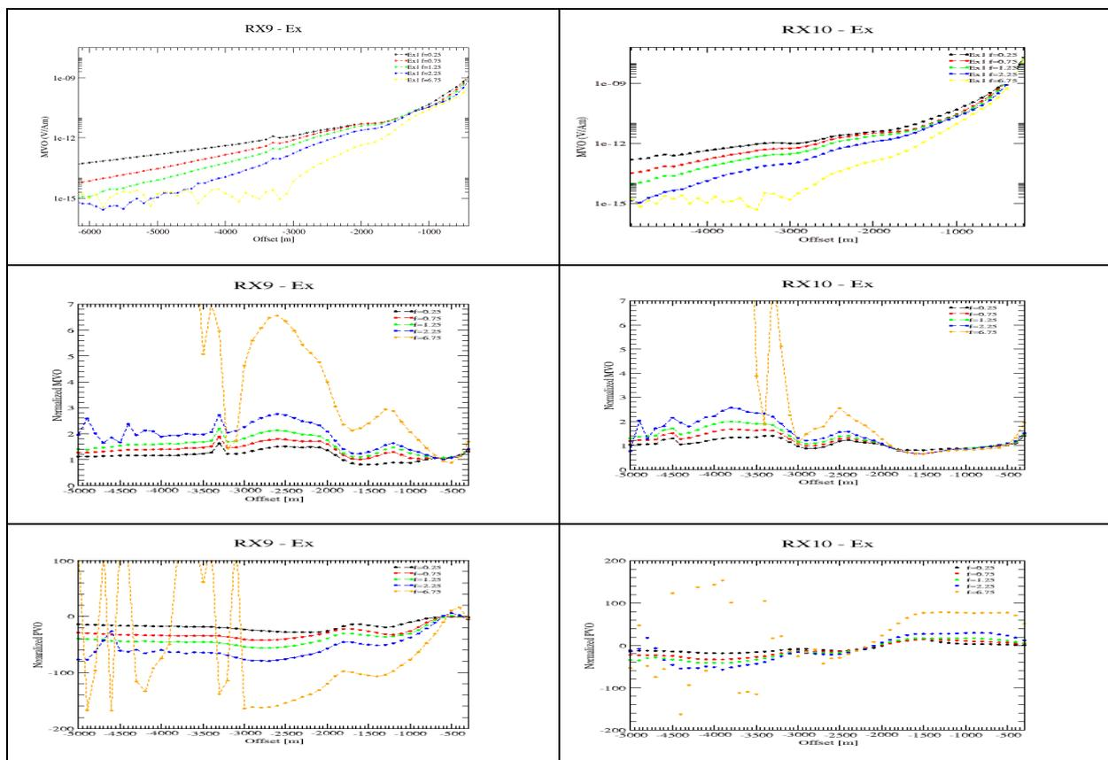
**Figure 3.** Ex - data from two receivers from a recent deep – water SBL survey: RX9 (LHS) and RX10 (RHS), respectively, see also RHS in Figure 2. Plots for different frequencies: 0.25Hz (black), 0.75Hz (red), 1.25Hz (green), 2.25Hz (blue), 6.75Hz (yellow). Upper panel: non – normalized MVO plots. Center panel: normalized MVO plots. Bottom panel: PVO – difference plots. The red boxes illustrating the locations of the methane hydrate patches are not exactly drawn to scale.
