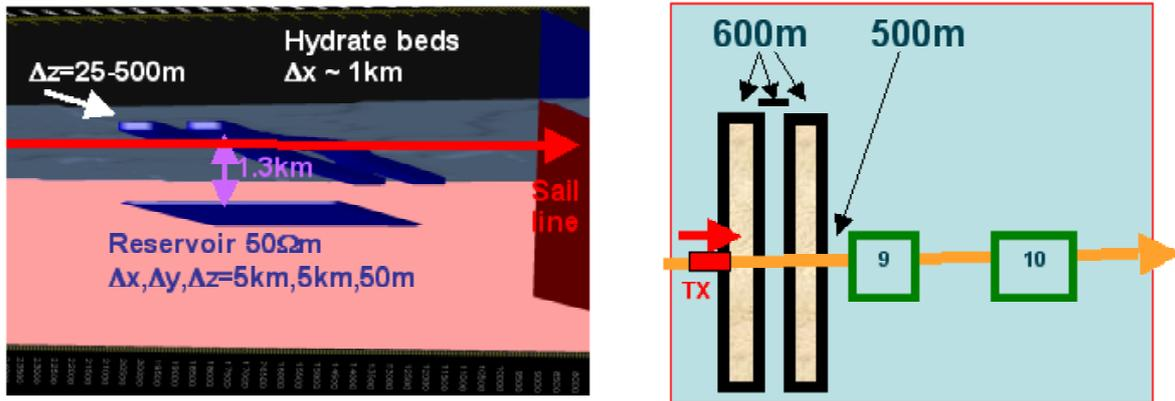
**Figure 2.** Left panel: illustration of hydrate patches with a characteristic length scale of ~1 km at a 1.7 km water depth above a synthetic target reservoir. Right panel: Top view of hydrate patches with the location of the receivers RX9 (“9”) and RX 10 (“10”) with 1.25km spacing.
