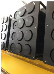
Figure: IGBT A Module
